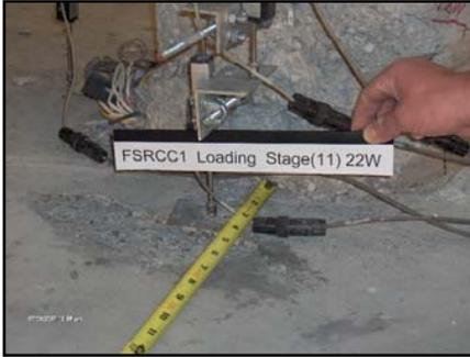
Figure 13 Minor Cracks on the Slab Surface
