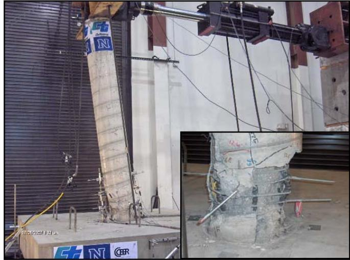
Figure 14 Specimen FSRCC1 During Last Stage
